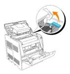
3. Grab the drum cartridge by the handle, and pull it up and out.
