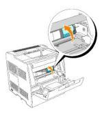
3. Hold the toner cartridge and pull out the cartridge.
