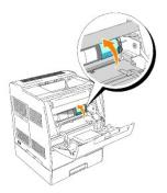
3. Hold the toner cartridge and pull out the cartridge.
