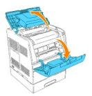
2. To remove the used drum cartridge, push up the lever on the right side of the printer.
