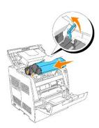
6. Pull down the lever on the right to lock the drum cartridge in place.
