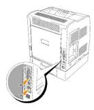
4. Hold the bottom of the multi protocol card and remove it from the control board.
