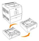
6. Place the printer on top of the standard 250-sheet tray module.
